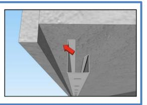
2. In order to attach the channel to the surface there are two common methods; 1. Use a screw through the back of the channel (As shown in diagram) penetrating into the frieze board. 2. Use a screw going vertical passing through one of the diode holes in the channel and penetrating through the lip of the channel on the top. And anchoring into the structure above.
